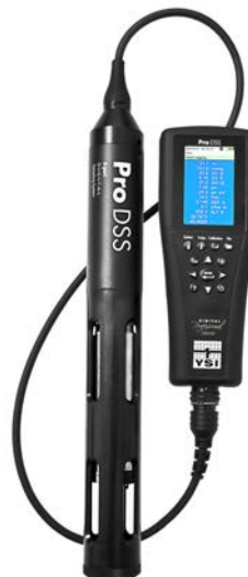
The YSI ProDSS features depth, GPS, optical DO, and many other sensors that are ideal when completing a lake profile.
