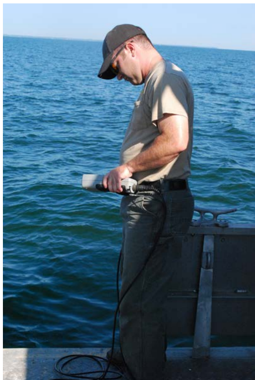
A Great Lakes Fisheries Biologist uses a YSI 556 on Lake Erie during a previous survey. The ProDSS is now the standard instrument used when collecting this data.
